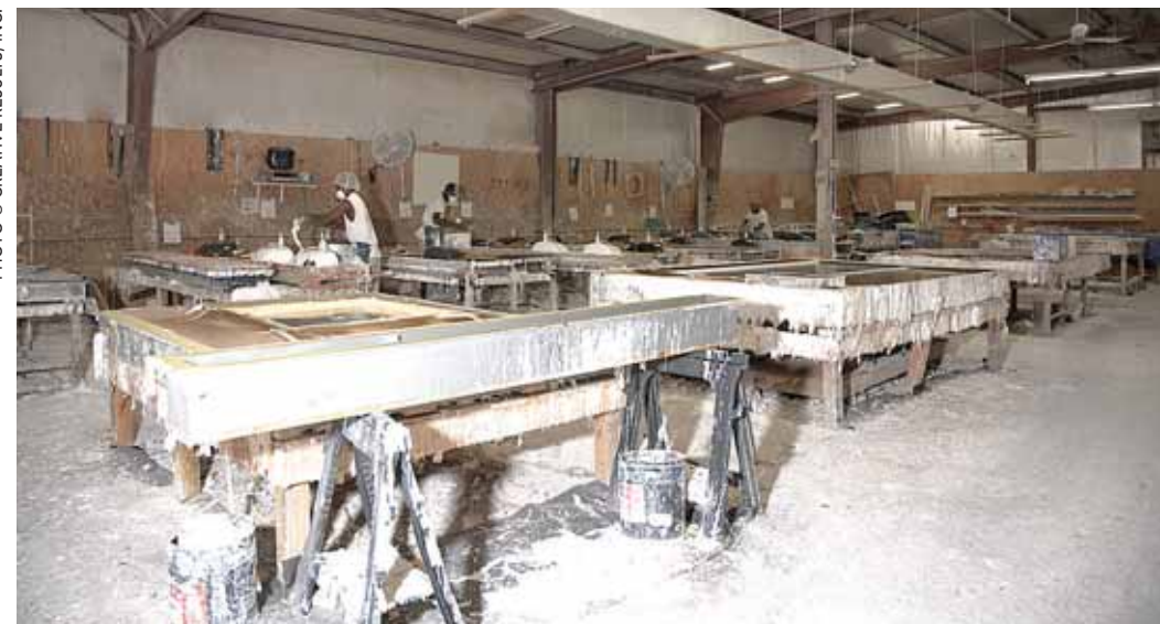
Easton Industries has manufactured cultured marble and Eastonite the same way since 1974. Pouring each custom piece by hand.
